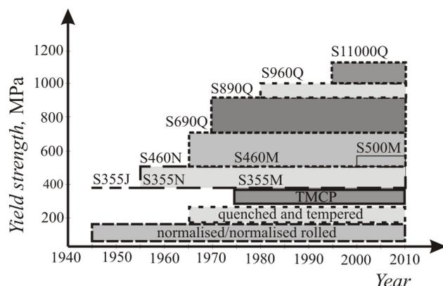
Fig.3. The evaluation of general purpose constructional steels and its yield strength
