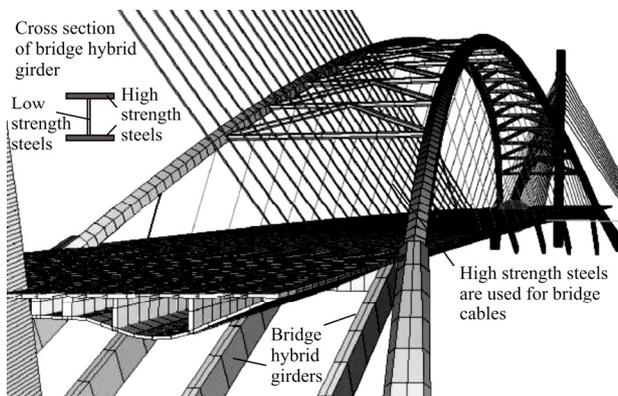
Fig. 8. Bridge design with hybrid girders
