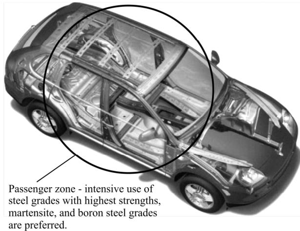
Fig.4. Steel grades at passenger zone of car body made to resist deformation and provide passive safety
