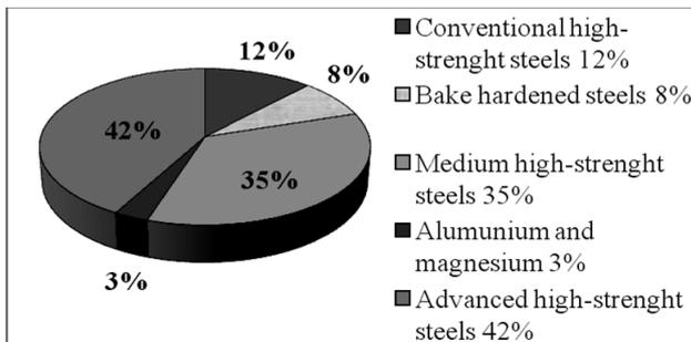
Fig.12. The projections for materials shares in 2015 year at mechanical constructions
