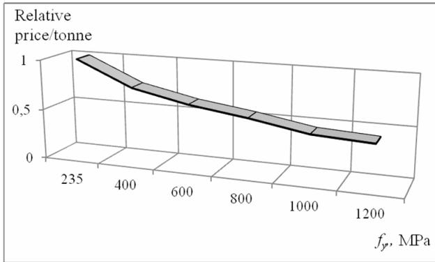
Fig. 7. Approximate referent price of high strength steels on the basis of load capacity
