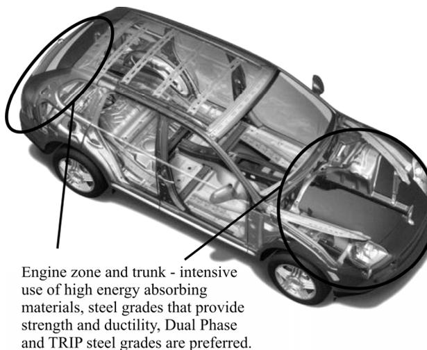
Fig.5. Steel grades for energy management zones of car body made to deform for absorb energy in collision
