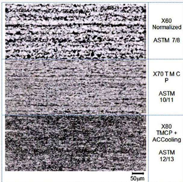
Fig.1. Typical microstructure and grain refinement in different high strength steels grades [2]
