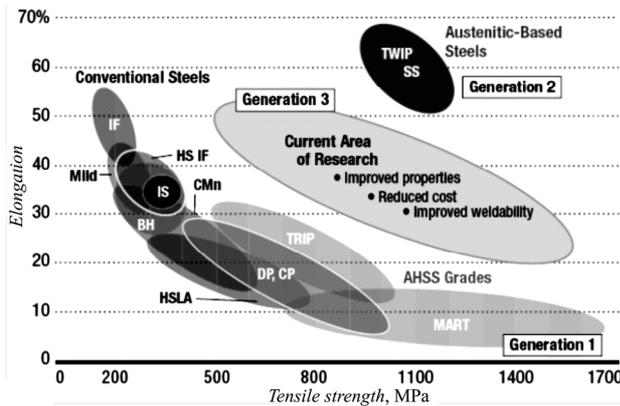
Fig.10. The generations of high strength steel grades and its basic mechanical properties
