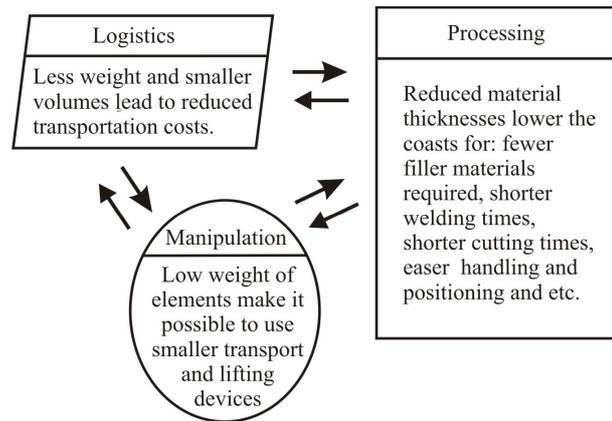
Fig. 9. Savings at different production stages provided by application of high strength steels
