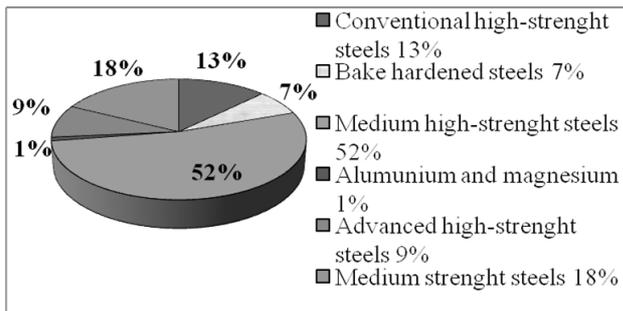
Fig.11. The materials shares for application at present mechanical constructions
